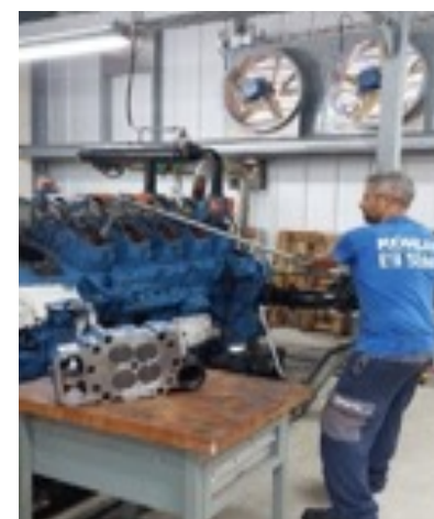
Long shot job needing the presence of our technicians on site during a few weeks and several rotations. Here torque tightening of a cylinder head screw with a long handle wrench.
