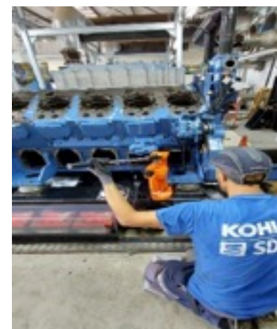
And here the operator is changing the engine damping pad, using a hydraulic jack to lift the engine from the chassis.
